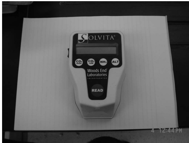
Figure 10. DCR digital reader for CO 2 -C analysis.
