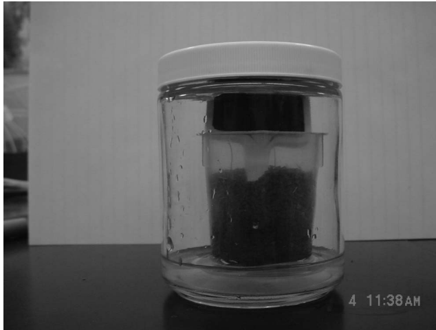
Figure 8. Soil and Solvita paddle enclosed in glass jar ready for incubation.
