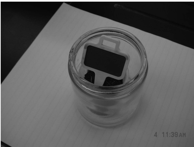
Figure 7. Solvita paddle in soil with glass jar.
