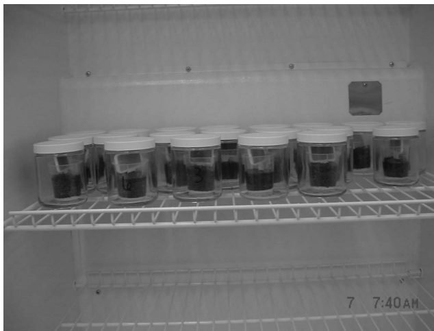
Figure 9. Incubated soil samples using the Solvita gel paddles for 24 h CO 2 -C analysis.
