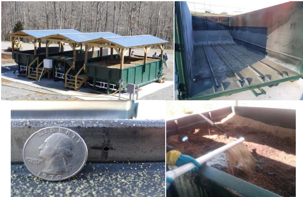
Figure 2. Forced Air System and Its Components. Forced air system ( top left ); rolloff container with stainless steel aeration tubes ( top right ); air hole on side of aeration tube ( bottom left ); and leachate hose used to wet compost with leachate pumped from collection tank ( bottom right ).
