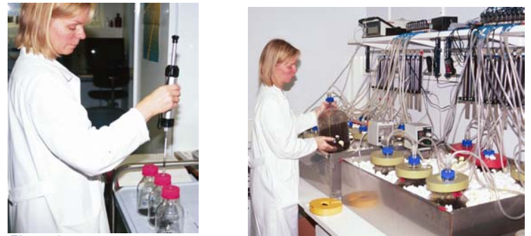
Figure 3. VTT CO 2 test and ASTM O 2 consumption test.
