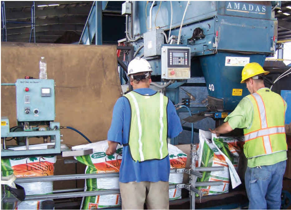
Bagging is done on-site using two Amadas electric bagging lines complete with palletizers (above). Leafgro® is sold in 1.5 cubic foot bags (right), as well as in bulk.
