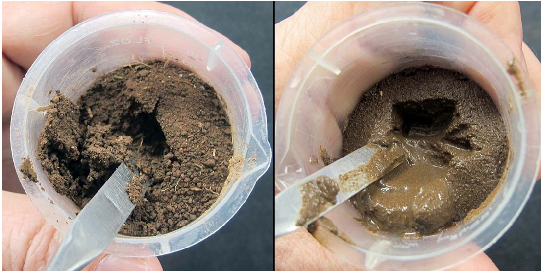
Figure 1. (Left) A well-structured soil wetted from below and unstructured soil (right) with same treatment. The soil on the left was processed at 2mm sieving and the soil at right is from a soil proficiency program which homogenizes samples to 0.7mm-minus.
