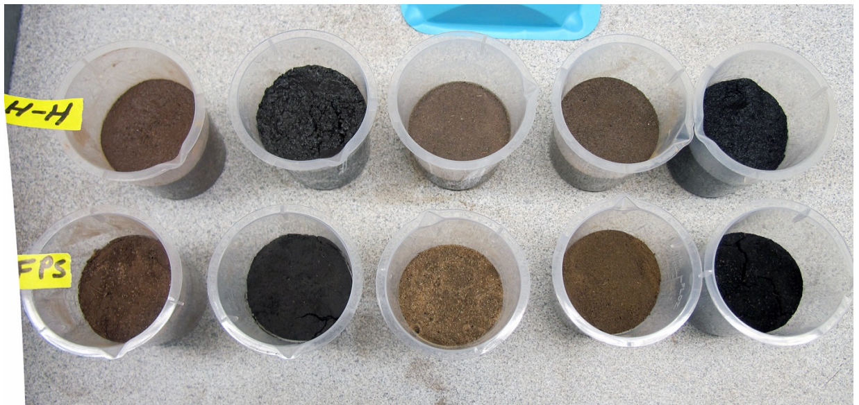
Figure 2. The five ALP samples used in the test runs, after wetting. Top Row after Standard method capillary wetting and lower row after 50% WFPS wetting. A spatula is required to open the surface to detect excess water in the over wet samples.
