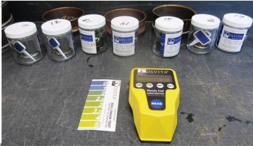
Figure 2 – Color Reference Chart, Digital Color Reader, Beakers, Jars and Gel Paddles
