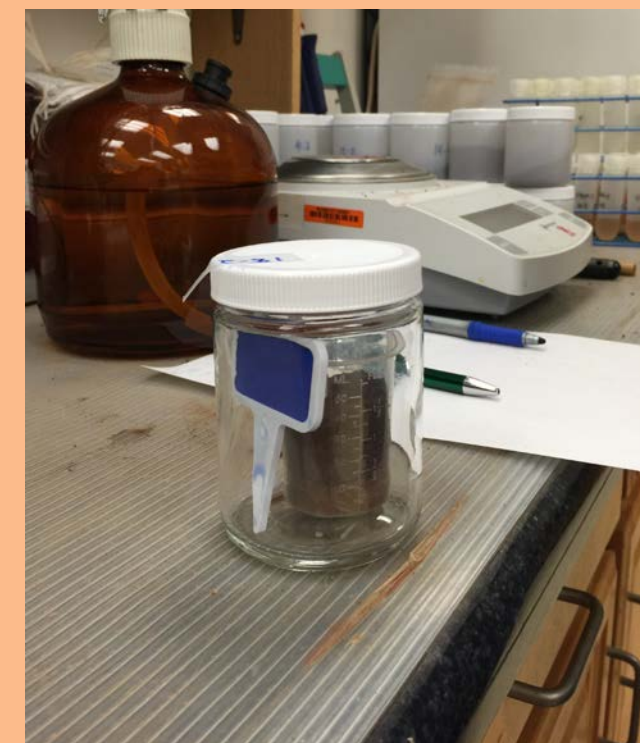
Picture 2: Completed setup of Solvita Jar, CO2 paddle included
