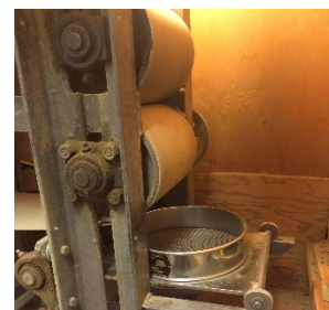
Fig 2. Early Soil Roller still in use (Univ. Maine Soil Lab)
