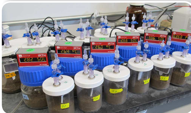
Two different infrared (IR) methods were employed to validate Solvita response in situ: Solvita jars affixed with gas sample ports for IR (front row); and "IRTH" jars with IR and Solvita inside the same jar.
