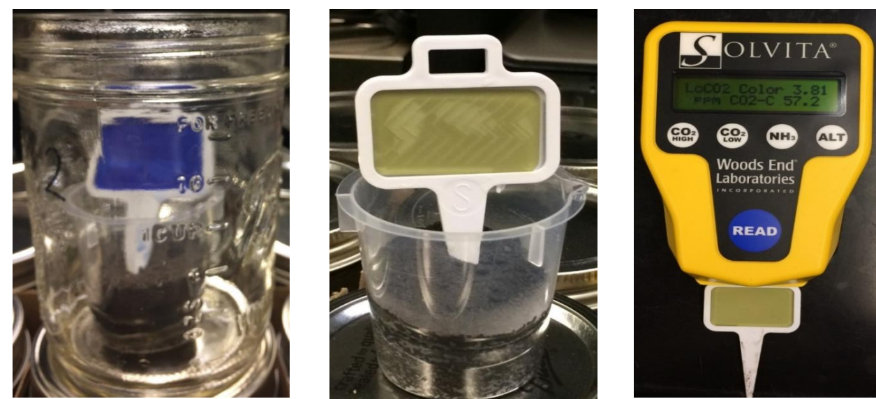
Fig. 2. Measuring soil CO 2 respiration using the Solvita technique (CO 2 -C evolved during 24-h incubation at uniform water content).
