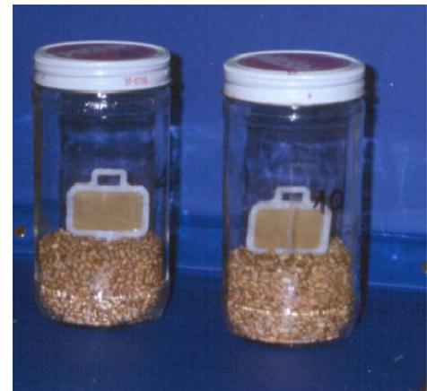
Figure 1. One pint jars containing shelled corn samples and CO<sub>2</sub> indicator paddles.
